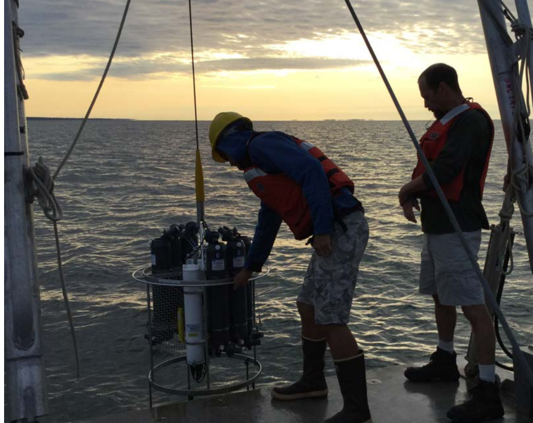
Chris Mills, a UConn student and crew member of the R/V Lowell Weicker, prepares to deploy a CTD rosette water sampler filled with Niskin bottles into Long Island Sound as Dave Cohen, marine technician, looks on. Photo: Judy Benson
