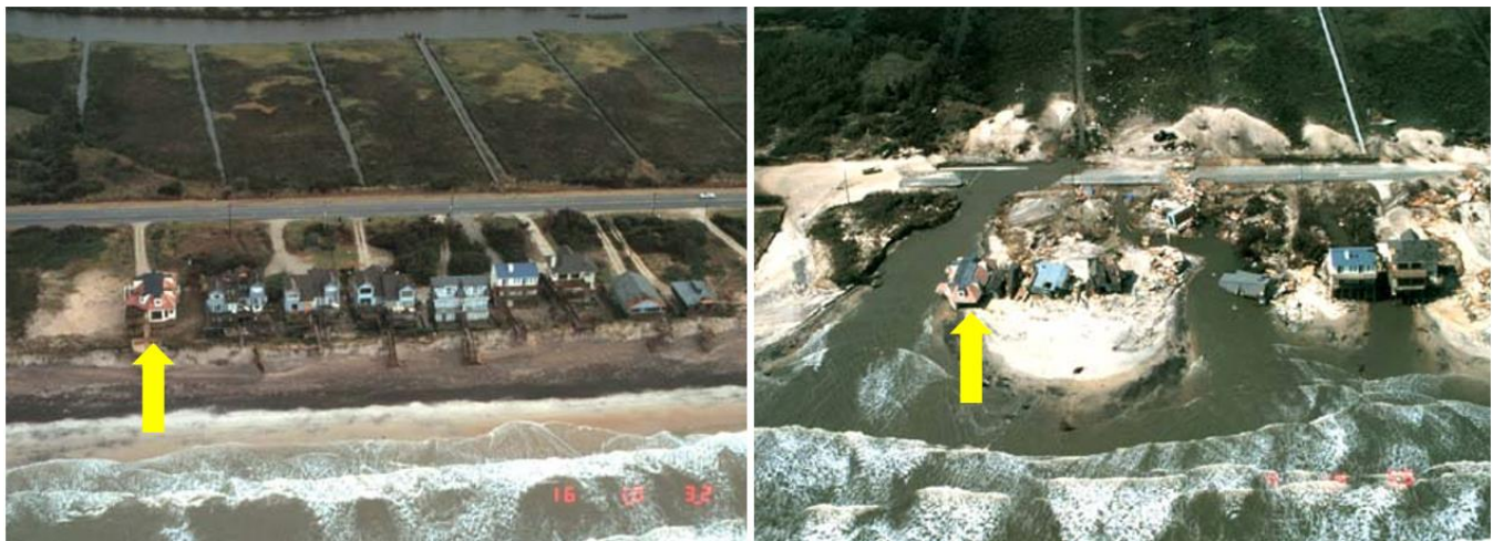
Figure 2. Before and after photos of hurricane Fran (1996) impacts on NTB. Yellow arrow indicates the same home in both images. Photo credit USGS (modified slightly).
